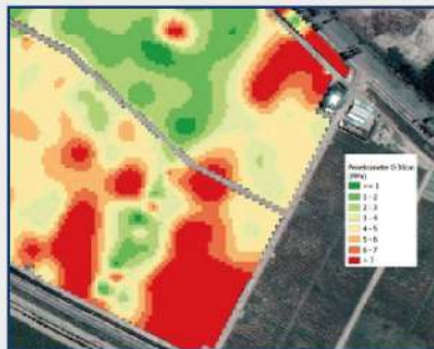
Average penetration resistance from 0 to 30 cm depth, Finca Santa Rosa, Santa Rosa, Mendoza.
