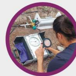
Scholander pump recording water potential measurements at solar noon.
